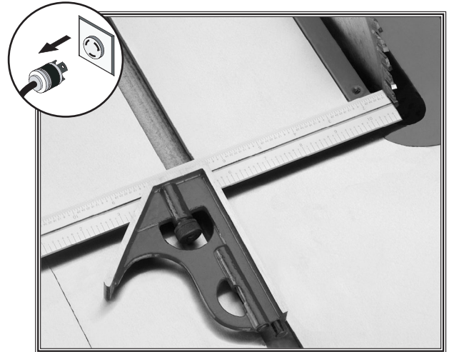
Figure 70. Example of adjusting blade to miter slot.
